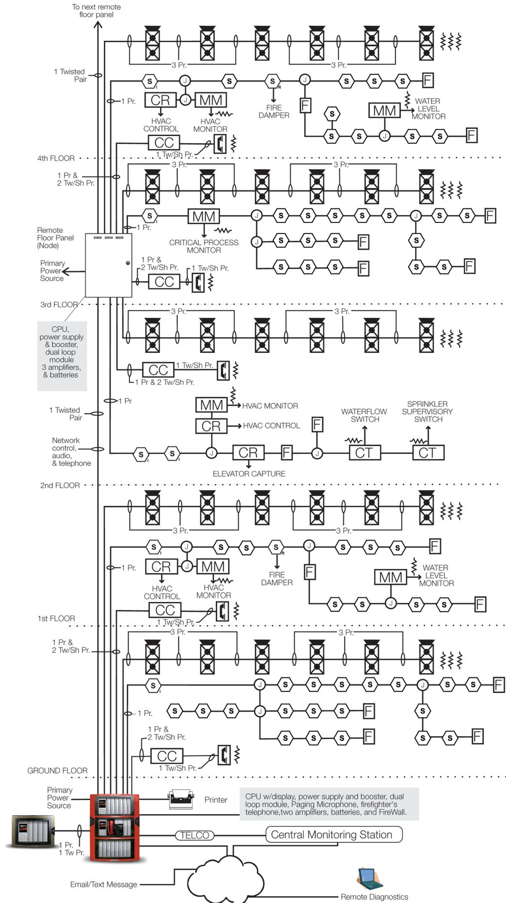
System design benefits greatly from this huge capacity. Minimal cabling requirements take scalability a step further. With EST4 a single copper pair or single fiber supports panel network data, audio data, as well as telephone data. This cuts cable counts by up to 75 per cent. Meanwhile, multiple firefighter's telephones risers are accommodated on the network, which allows them to be deployed at much further distances compared with analog audio transmission methods.
