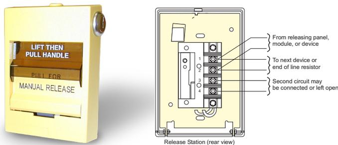
The manual release station is a normally-open, dry contact signal initiating device. The 276A-REL is a single-action station that requires the user to pull the release handle to initiate the release of a fire suppression agent. The 278A-REL (shown) is a double-action station that requires the user to raise the upper door, then pull the release handle to initiate the release.
