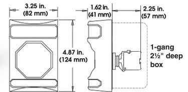
The abort station is a normally-open, non-latching device. It is used to prevent the release of agent into the protected area after the release sequence has begun.
